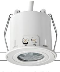
ambient light is at approximately the minimum desired working light level, a lux meter placed on the surface under the PIR may help. With the LUX set fully clockwise wait for the PIR to switch off. Rotate the LUX adjuster slowly anticlockwise (- to +), whilst waving your hand approximately 1m below the PIR, until the load switches on.
